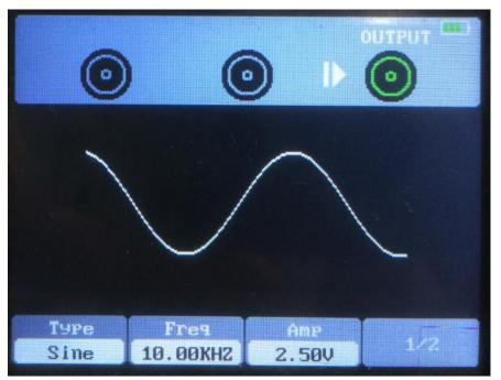
6. Press D button, the backlight of the button turns green, i.e. output sine waveform.
